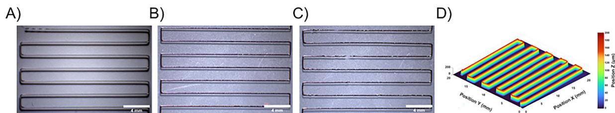
**Fig. 6** Stereomicroscopy images of (A) PCL, (B) PCL-P3HT-1 and (C) PCL-P3HT-4 digital snakes printed using the 120 °C\_700 kPa\_4 mm s<sup>-1</sup> parameters. Scale bars are 4 mm. (D) Profilometry 3D mapping of the sample presented in (A).
