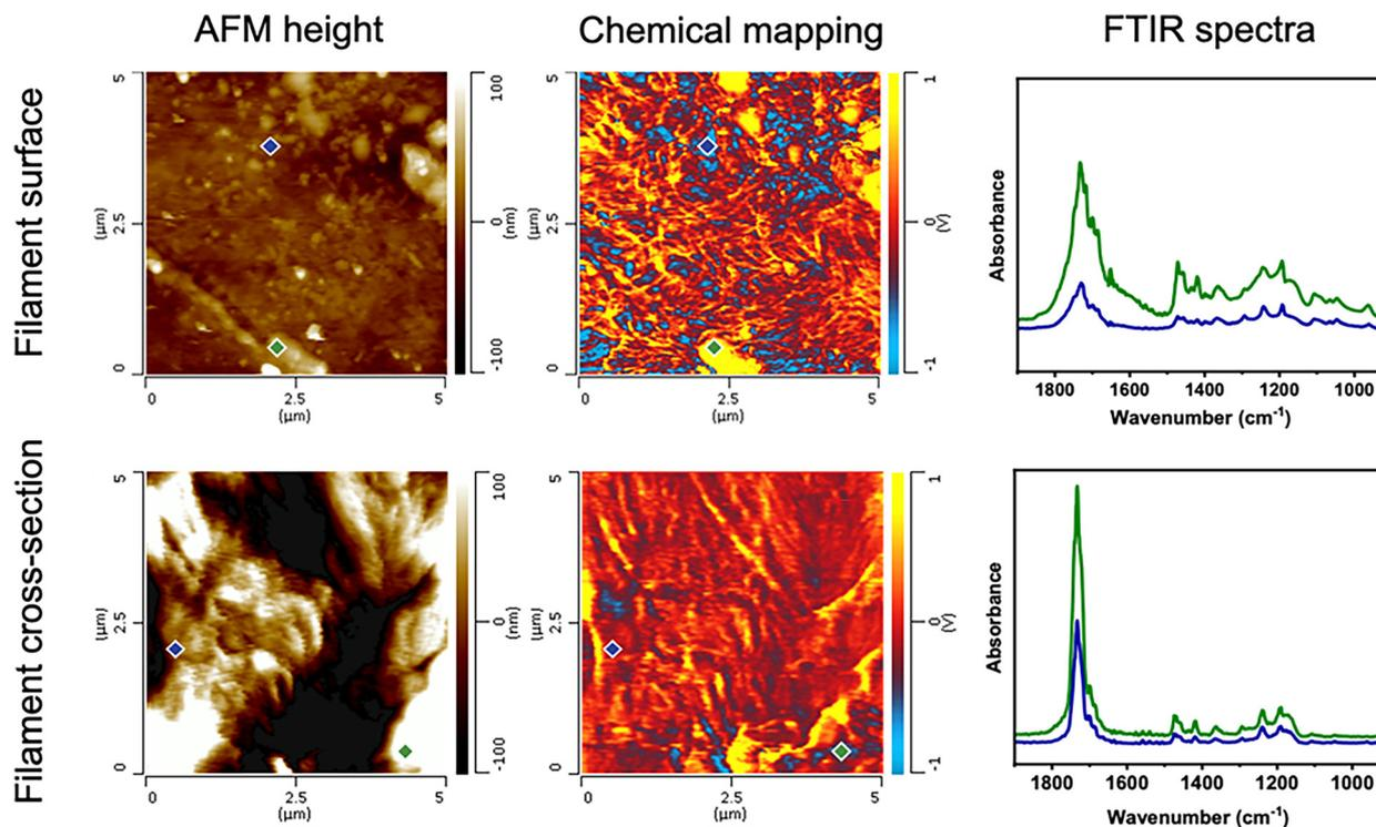
Fig. 8 AFM height images and chemical mapping at  $1732\text{ cm}^{-1}$  for PCL-P3HT-1 (printed at  $120\text{ }^{\circ}\text{C}$  and  $700\text{ kPa}$ ) on the filament surface or its cross-section. Blue and green dots on these images represent the location where the FTIR spectra are taken.
