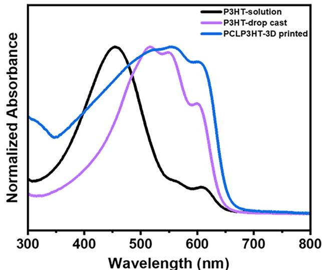
Fig. 7 Transmission UV-visible spectra of a P3HT solution in  $\text{CHCl}_3$  and drop cast P3HT film combined with the diffuse reflectance UV-vis spectrum of PCL–P3HT-0.4 digital snake printed at  $140^\circ\text{C}$ .
