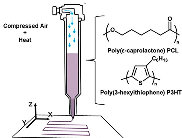
Fig. 1 Schematic illustration of the hot-melt extrusion of the P3HT-PCL blend.
