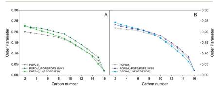
Fig. 2 Smoothed  $^2$ H NMR order parameter plots of symmetric and asymmetric MLVs determined from the  $^2$ H NMR spectra shown in Fig. 1. (A) Order parameters of POPC- $d_{31}$  and (B) order parameters of POPS- $d_{31}$  are plotted. The temperature of the measurement was 37  $^{\circ}$ C.
