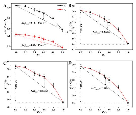
Fig. 4 Compositional dependence of (A) longitudinal sound velocity ( $\nu_L$ ) and transversal sound velocity ( $\nu_T$ ), (B) Young's modulus E, (C) Bulk modulus Eand (D) Shear modulus G at room temperature as a function of the molar ratio R (R is equal to the molar ratio of  $[K_2O]/([Na_2O] + [K_2O]))$
