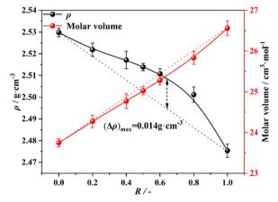
Fig. 5 Compositional dependence of the density  $(\rho)$  and molar volume of the  $65.0 \text{SiO}_2 \cdot 5.0 \text{B}_2 \text{O}_3$  (17.6 - x)·Na<sub>2</sub>O·xK<sub>2</sub>O·7.5CaO·4.9MgO glasses as a function of different molar ratios R, where R is equal to the molar ratio of  $[K_2O]/([Na_2O] + [K_2O])$ . The dashed line is a guide for the eye.
