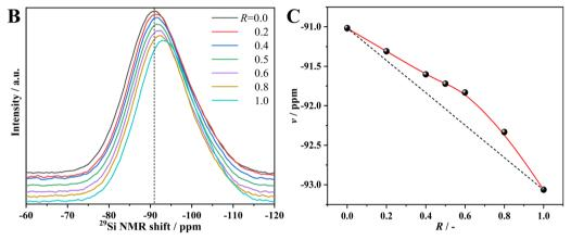
Fig. 6 (A)  $^{11}$ B NMR spectra of the 65.0SiO<sub>2</sub>·5.0B<sub>2</sub>O<sub>3</sub> (17.6 – x)·Na<sub>2</sub>O·xK<sub>2</sub>O·7.5CaO·4.9MgO glasses, where R is equal to the molar ratio of  $[K_2O]/([Na_2O] + Na_2O)/([Na_2O] + Na_$ [K<sub>2</sub>O]). (B)  $^{29}$ Si NMR spectra of the glasses with different R. (C) Dependence of the peak position ( $\nu$ ) near -91 ppm as a function of the molar ratio R. Dashed line: the linear correlation between the two endmembers.
