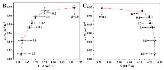
Fig. 3 Relationship between thermal conductivity (k) and (A) Debye sound velocity ( $\nu_D$ ), (B) volumetric heat capacity (C) and (C) phonon mean free path (t) for the glasses with different R investigated in this work. The dashed line is a guide for the eye.
