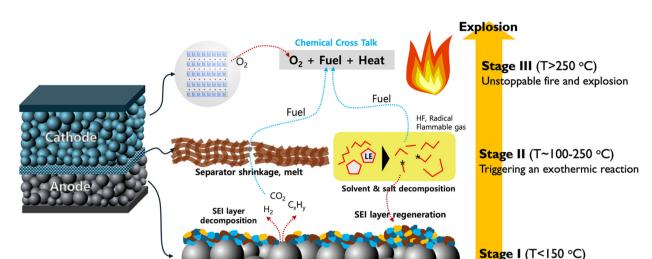
Schematic illustration of the sequence of events during thermal runaway
