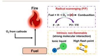
Fig. 4 General strategies for flame-retardant or non-flammable electrolytes.
