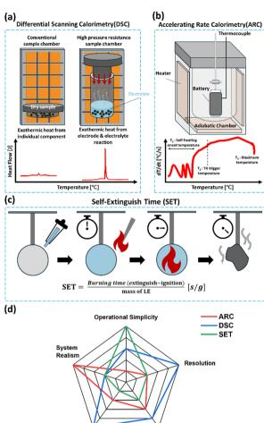
Fig. 3 Schematic diagrams of typical thermal analysis tools (a) DSC, (b) ARC, and (c) SET. (d) A radar chart comparing their characteristics.
