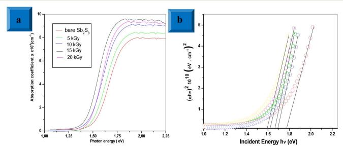
Fig. 12 UV-vis absorption spectra for bare and irradiated  $Sb_2S_3$  thin films at different doses (a). Tauc plot for bare and irradiated samples was obtained from the absorption spectra; the solid lines represent the linear regressions on the data from which the optical band gap energies were determined (b).
