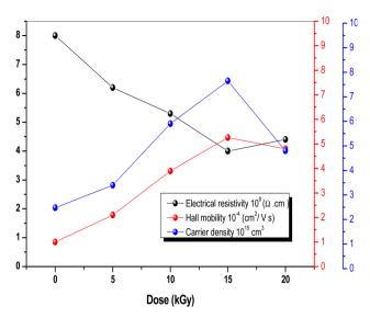
Fig. 11 Electrical resistivity, Hall mobility, and carrier density of  $Sb_2S_3$  thin films before and after  $\gamma$ -irradiation with different doses.
