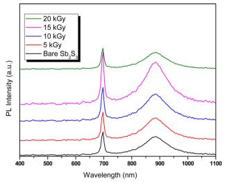
Fig. 13 Photoluminescence (PL) spectra of Sb<sub>2</sub>S<sub>3</sub> thin films before and after γ-irradiation with different doses.
