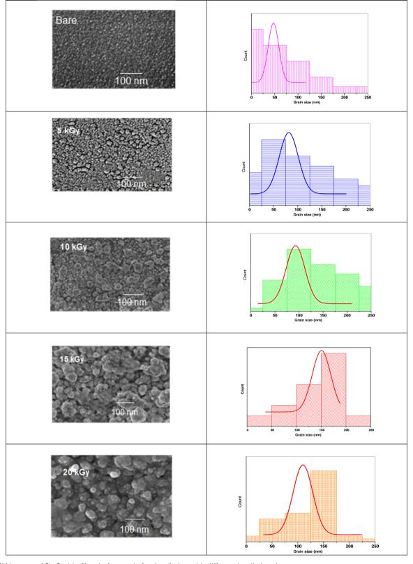
Fig. 9 SEM images of  $Sb_2S_3$  thin films before and after irradiation with different irradiation doses.
