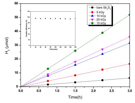
Fig. 18 Hydrogen evolution as a function of time for different  $Sb_2S_3$ -based photocathodes under standard one sun (100 mW cm<sup>-2</sup>) illumination at 0 V vs. RHE. The inset plot of Fig. 15 stands for the faradaic efficiency (FE) measurement of the optimized  $Sb_2S_3$ -based photocathode (15 kGy).
