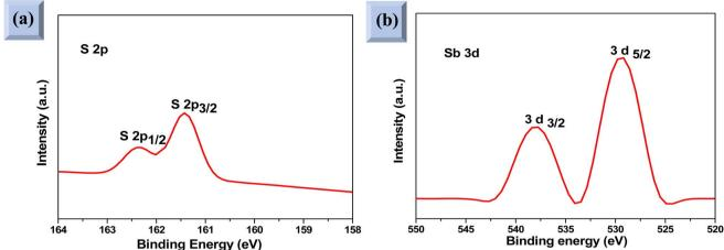
Fig. 4 High-resolution XPS spectra of (a) S 2p and (b) Sb 3d core levels of the bare  $Sb_2S_3$  material.
