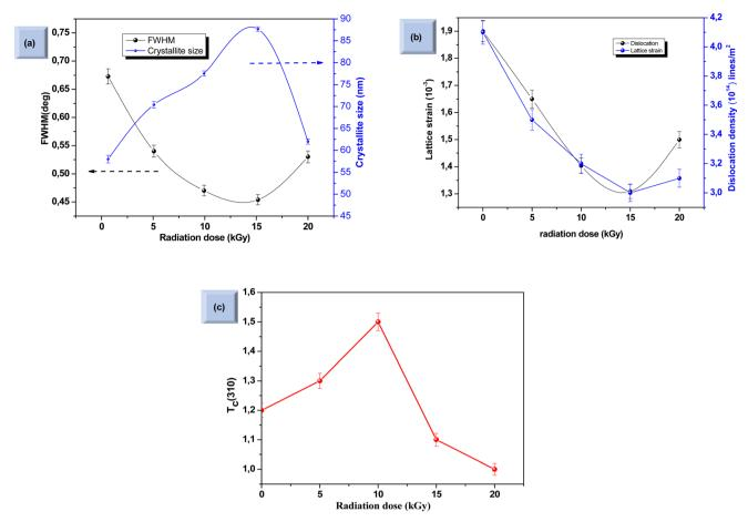
Fig. 7 Variation of full width at half maximum (FWHM) and crystallite size as a function of irradiation doses (a). Variation of dislocation density ( $\delta$ ) and lattice strain at different irradiation doses (b). Influence of  $\gamma$  radiation on texture coefficient  $T_c$  (310) (c). Each data point in the two graphs is accompanied by error bars that represent a 2% margin of uncertainty and provide a quantifiable measure of the variability in our measurements.
