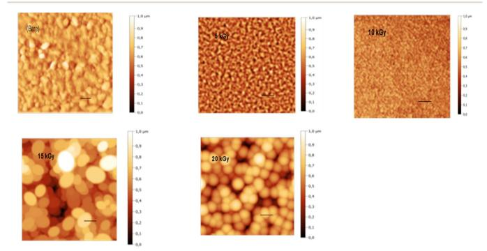
Fig. 10 2D AFM micrographs of bare and irradiated Sb<sub>2</sub>S<sub>3</sub> thin films at different doses. The scale bar on all images indicates a length of 100 nm.
