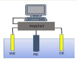
Fig. 2 Illustration for the three-electrode setup used in the photo-electrochemical technique. WE = working electrode (Sb<sub>2</sub>S<sub>3</sub> thin films); RE = reference electrode (SCE); CE = counter electrode (Pt plate).
