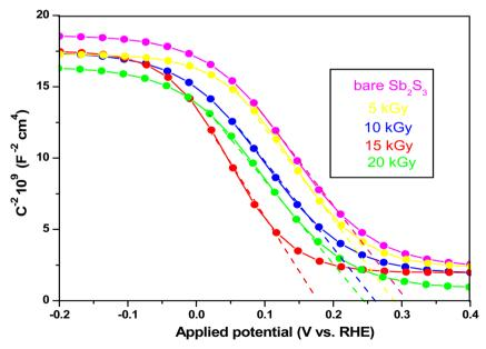
Fig. 16 Mott–Schottky plots of bare and irradiated Sb<sub>2</sub>S<sub>3</sub>-based photocathodes.
