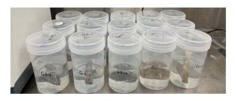
Fig. 1 Experimental setup for LEAF 1315 with concrete monoliths suspended in DI water.
