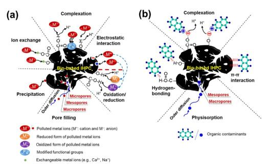
Fig. 5 Working mechanisms for the removal of (a) metal ions<sup>11,19,56,126–129</sup> and (b) organic compounds<sup>2,57,123,132</sup> via bio-based IHPCs.
