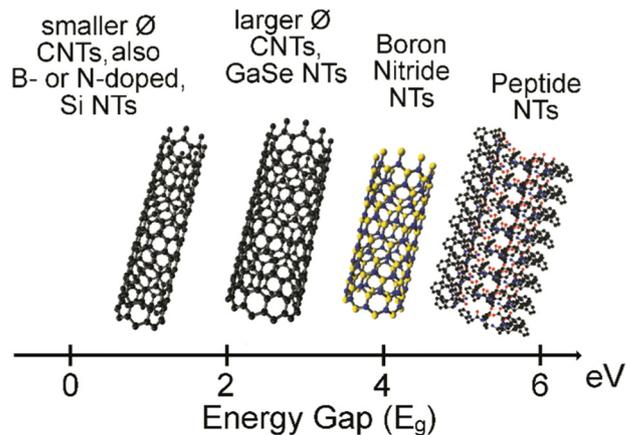
Fig. 1 HOMO–LUMO energy band gap in electronvolt (eV) for CNTs, inorganic NTs, and peptide NTs.<sup>16,17</sup>
