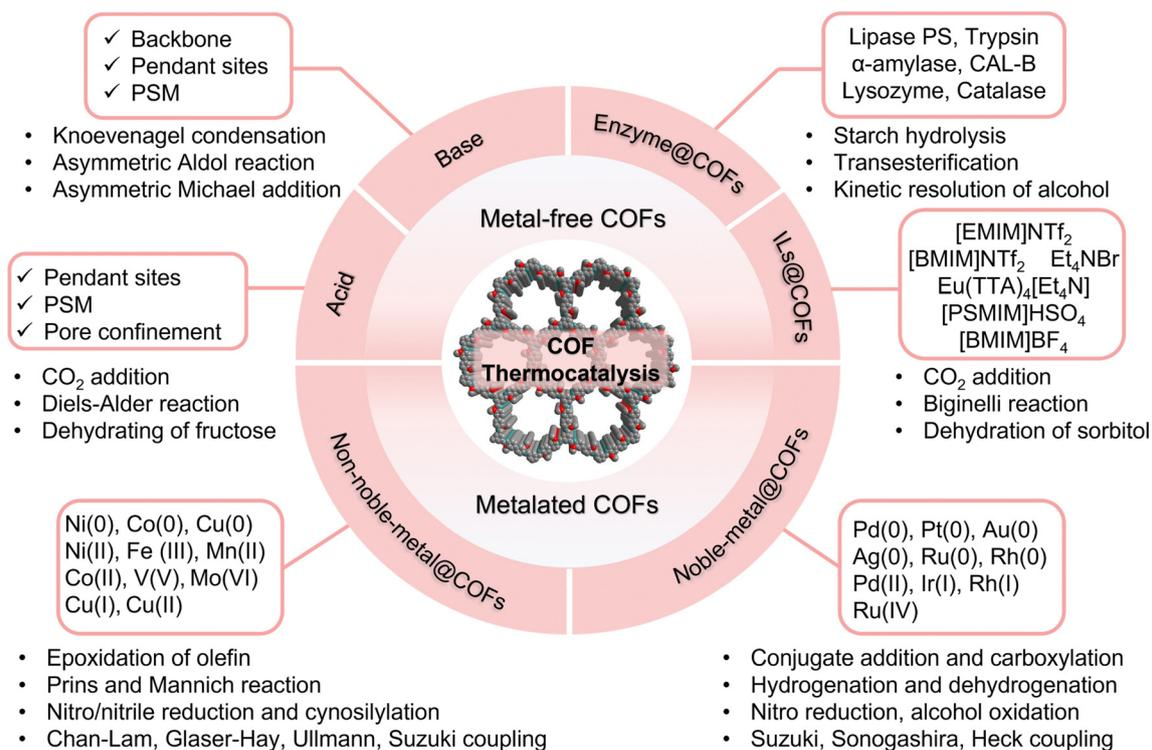
Scheme 3 Leading design strategies and notable examples of COF catalysts for thermocatalysis.
