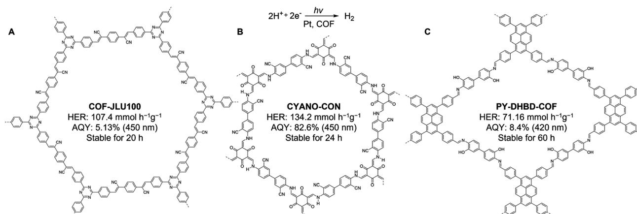
Fig. 8 Schematics of (A) sp<sup>2</sup>c-COF-JLU100, (B) CYANO-CON, and (C) *in situ* Pt-PY-DHBD-COF for visible-light-driven HER.
