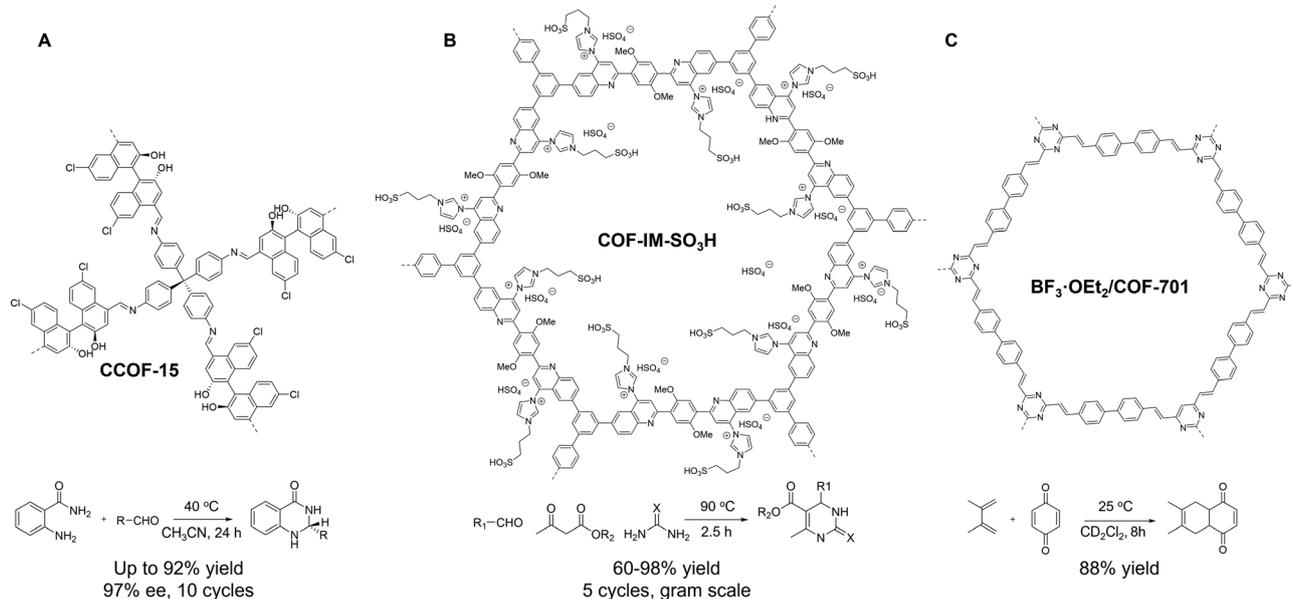
Fig. 2 Schematics of (A) 3D CCOF-15 with chiral acidic linkers, (B) COF-IM-SO<sub>3</sub>H made *via* PSM, (C) BF<sub>3</sub>·OEt<sub>2</sub>/COF-701 as solid acids for thermocatalysis.
