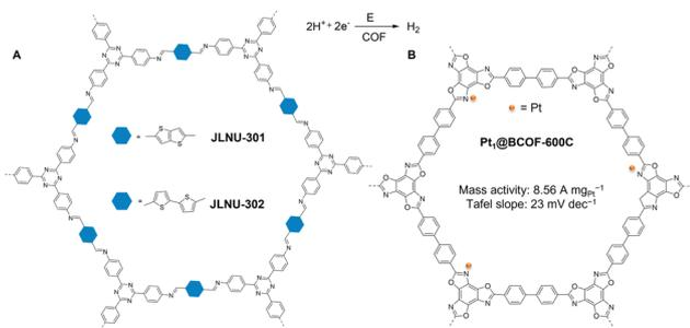
Fig. 10 Schematics of (A) JLNU-301 and -302; (B) single-atom Pt<sub>1</sub>@BCOF-600C for electrocatalytic HER in acidic media.
