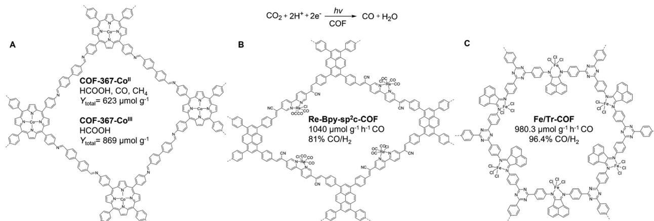
Fig. 9 Schematics of (A) COF-367-Co<sup>II</sup> and Co<sup>III</sup>, (B) Re-Bpy-sp<sup>2</sup>c-COF, and (C) Fe/Tr-COF for CO<sub>2</sub> photoreduction under visible-light irradiation.
