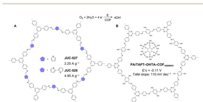
Fig. 11 Schematics of (A) JUC-527 and JUC-528, (B) PA/TAPT-DHTA-COF<sub>1000</sub>NH<sub>3</sub> electrocatalytic ORR in alkaline media.
