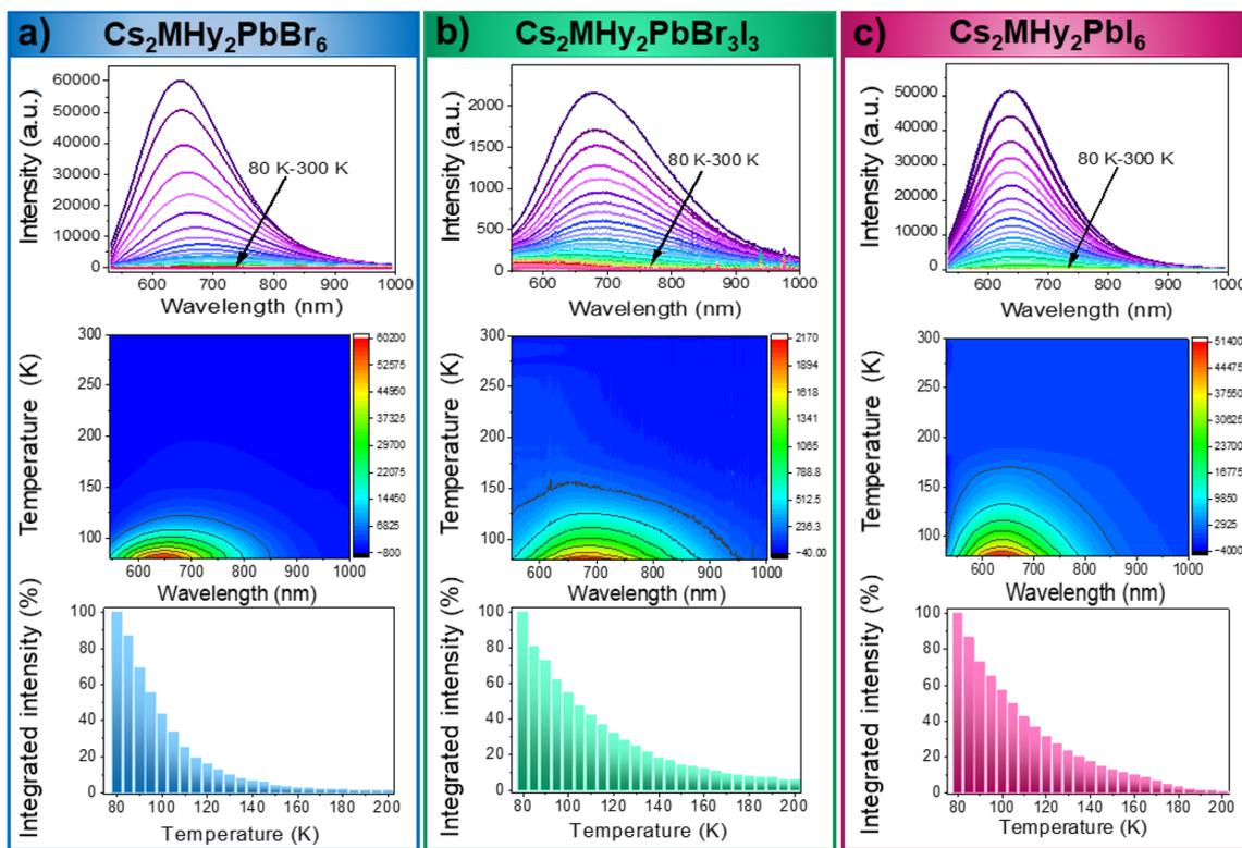
Fig. 6 Temperature-dependent emission spectra recorded from 80 to 300 K, the PL intensity contour map, and the integrated emission intensity at various temperatures of (a)  $\text{Cs}_2\text{MHy}_2\text{PbBr}_6$ , (b)  $\text{Cs}_2\text{MHy}_2\text{PbBr}_3\text{I}_3$ , and (c)  $\text{Cs}_2\text{MHy}_2\text{PbI}_6$ , respectively.
