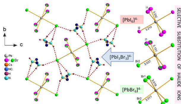
**Fig. 2** The N–H...Br HB network in  $\text{Cs}_2\text{MHy}_2\text{Pb}(\text{Br}/\text{I})_6$ . In each  $\text{Pb}(\text{Br}/\text{I})_6$  there are two sites for halogen ions interacting with middle-chain  $\text{NH}_2^+$  groups. In  $\text{Cs}_2\text{MHy}_2\text{PbI}_3\text{Br}_3$  they are preferentially occupied by  $\text{Br}^-$ .
