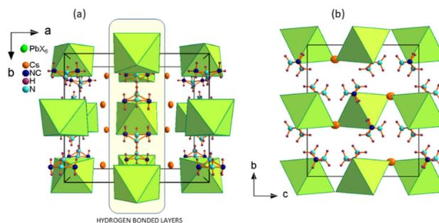
**Fig. 1** The crystal structures of Cs<sub>2</sub>MHy<sub>2</sub>PbX<sub>6</sub> and MHy<sup>+</sup> are disordered. (a) Discrete (0D) Pb (Br/I)<sub>6</sub> units interact through HBs with MHy<sup>+</sup> cations forming HB layers perpendicular to the *a* direction, coulombic interactions between caesium ions and Pb(Br/I)<sub>6</sub> units stabilize the structure perpendicular to the layers. (b) The view along the *a* direction.
