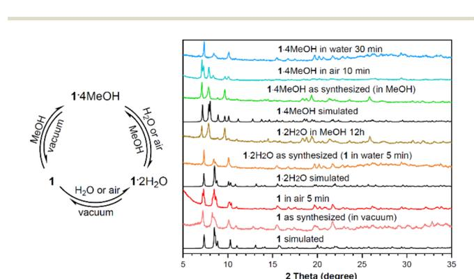
**Fig. 2** Reversible inter-conversions of **1**, **1**·2H<sub>2</sub>O and **1**·4MeOH, with PXRD patterns simulated from the SCXRD data and those of the samples during the inter-transformations.
