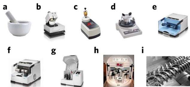
Fig. 3 Commonly used milling equipment. (a) Mortar and pestle, (b) automatic mortar, (c) vertical vibrational mini mill, (d) vibratory micro-mill, (e) vibrational ball mill, (f) vibrational ball mill with temperature control, (g) planetary ball mill, (h) multisampling mill, and (i) twin-screw for continuous mechanochemical synthesis. Reproduced with permission from ref. 15.
