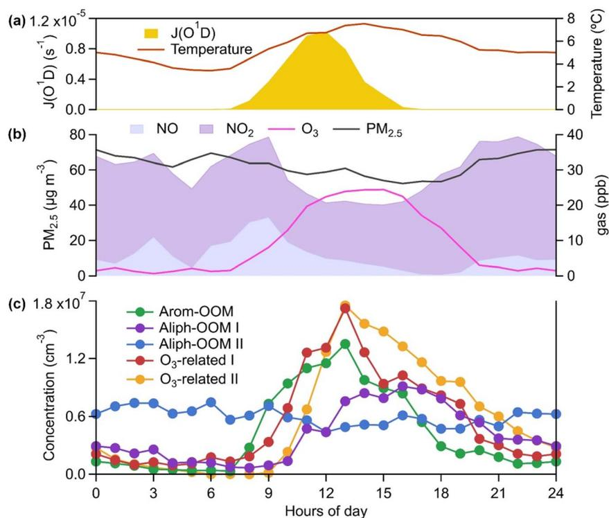
Fig. 1 Median diurnal variations of main compounds and parameters. (a)  $\text{NO}$ ,  $\text{NO}_2$ ,  $\text{O}_3$ , and  $\text{PM}_{2.5}$ . (b)  $J(\text{O}^1\text{D})$  and temperature. (c) The Arom-OOM, Aliph-OOM-I, Aliph-OOM-II,  $\text{O}_3$ -related-I, and  $\text{O}_3$ -related-II factors from binPMF analysis to OOMs.
