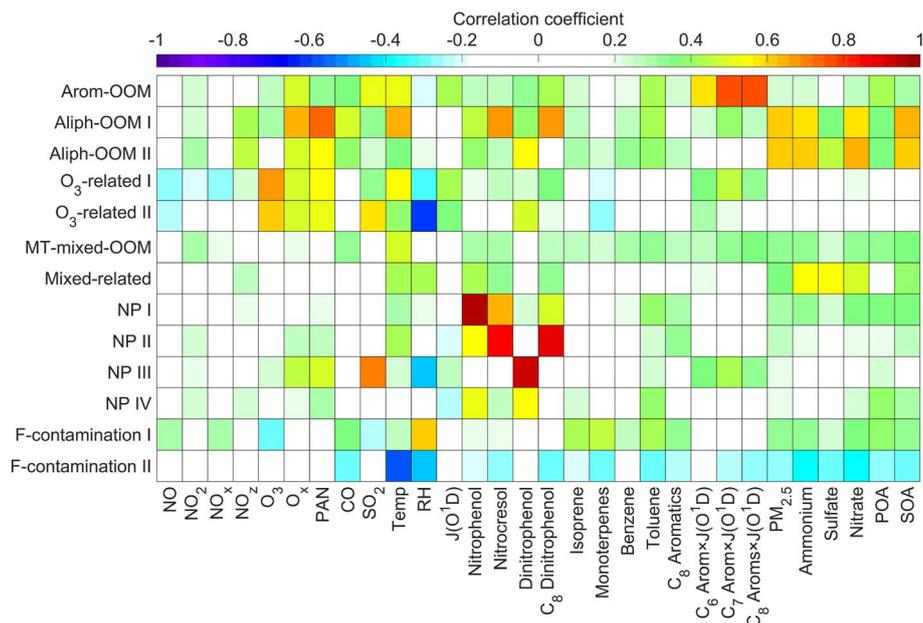
Fig. 4 Correlations of binPMF factors with external gas-phase and particulate tracers. The colors are differentiated by Pearson correlation coefficients. Note:  $O_x$  is the total oxidants ( $O_x = O_3 + NO_2 + NO_z$  and  $NO_z = NO_y - NO_x$ ); aromatics  $\times J(O^1D)$  are the proxies of aromatic photo-oxidation; and primary and secondary organic aerosols (POA and SOA) are derived from PMF analysis of the organic aerosol detected by TOF-ACSM.
