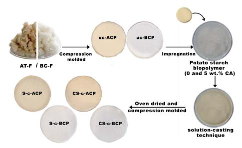
Fig. 2 Process of cellulosic papers preparation.
