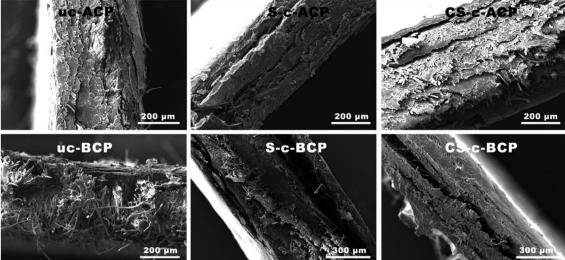
Fig. 6 SEM micrographs of the elaborated cellulosic papers cross-sections
