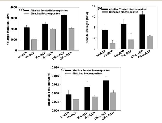
Tensile properties of the elaborated cellulosic papers.
