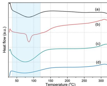
**Fig. 5** DSC thermograms (endotherm down) of the cured PPO<sub>900</sub>-Bz-Bor (a), and the 1<sup>st</sup> (b), 3<sup>rd</sup> (c) and 5<sup>th</sup> (d) cycles of the cured PPO<sub>900</sub>-Bz-Bor.
