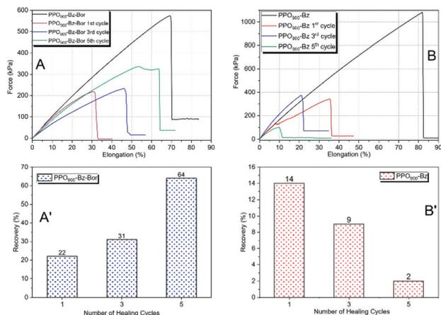
**Fig. 2** Stress–strain analysis of PPO<sub>900</sub>-Bz-Bor (A) and PPO<sub>900</sub>-Bz (B) and the healing efficiencies of PPO<sub>900</sub>-Bz-Bor (A') and PPO<sub>900</sub>-Bz (B').
