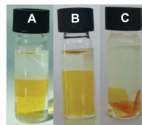
Fig. 7  $\text{PPO}_{900}\text{-Bz-Bor}$  in water for 1 (A), 5 (B), and 9 (C) days.
