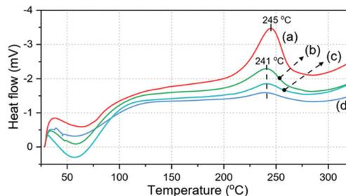
**Fig. 4** DSC thermograms (endotherm down) of PPO<sub>900</sub>-Bz (a), the cured PPO<sub>900</sub>-Bz (b), the cured PPO<sub>900</sub>-Bz after the 1<sup>st</sup> (c) and 5<sup>th</sup> (d) healings.
