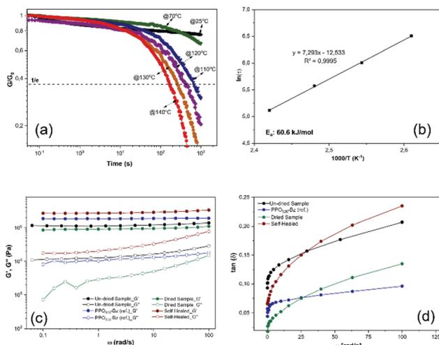
Fig. 6 Normalized relaxation module ( $G$ ) vs. time graphs for the cured  $\text{PPO}_{900}\text{-Bz-Bor}$  at different temperatures (a), the logarithm of relaxation time  $\ln(\tau)$  versus reciprocal temperature ( $1000/T$ ) (b), and the storage ( $G'$ ) and loss ( $G''$ ) moduli are plotted as a function of frequency for the samples of dried, undried, self-healed  $\text{PPO}_{900}\text{-Bz-Bor}$ , and  $\text{PPO}_{900}\text{-Bz}$  at 25 °C (c) and (d).
