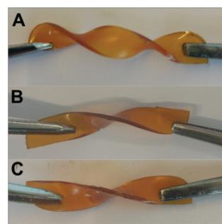
Fig. 1 Images of the cured PPO<sub>900</sub>-Bz-Bor film before healing (a), after the 3<sup>rd</sup> healing cycle (b) and the 5<sup>th</sup> cycle (c).
