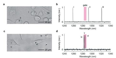
Fig. 6 Band-pass sorting. a, A bright-field image of replated cells collected from the (–) outlet. b, The LP lasing emissions from the LPs labelled i, ii and ii. c and d, Image and emission spectra of cells collected from the (+) outlet, showing three LPs (iv-vi).
