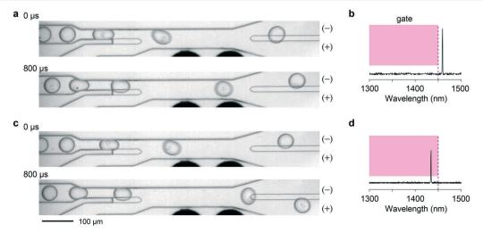
Fig. 5 Short-wavelength sorting, a, A negative cell (l > 1450 nm) flowing into the (-) channel, b, The LP emission spectrum of the negative cell. The magenta box indicates the gating condition used. c, A positive cell ( $\lambda$  < 1450 nm) directed into the (+) channel. d, The LP spectrum of the positive cell.
