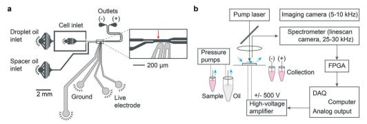
Fig. 2 The microfluidic system. a, Schematic of a microfluidic chip. Pump laser focus location shown in inset (red arrow). b, Schematic of the cell sorting setup. A spectrometer reads LP laser emission. Decision hardware in a field programmable gate array (FPGA) triggers the computer to send high voltage pulses to electrodes to deflect cell-containing droplets into the (+) outlet.
