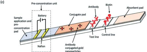
Fig. 2 Schematic illustrations of enhancement methods for hCG LFAs. (a and b) Test principle of a sandwich hCG LFA (a) before and (b) after enhancement using gold nanoparticles. (c) LFA and pre-concentration unit.
