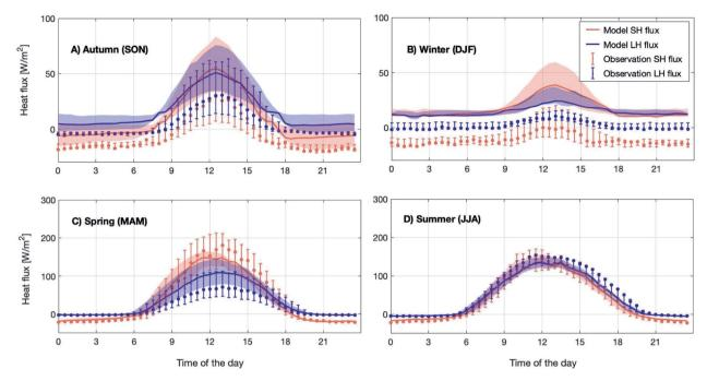
Fig. 1 Measured (dots) and modelled (solid lines) diurnal median sensible (SH, red) and latent (LH, blue) heat fluxes above the SMEAR II station (23 m) averaged for four seasons over the period 2007–2018 in subplots (A-D). The letters in brackets in the subplot titles represent the months used for the individual seasons. The 25<sup>th</sup>-75<sup>th</sup> percentile is shown as shades and vertical bars for modelled and measured fluxes, respectively.
