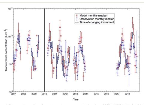
Fig. 4 Measured and modelled monthly median values of monoterpene concentrations from 2007 to 2018 for the height interval 32–125 m. The measurement median data were obtained from the mean values of five measurement heights: 32 m, 54 m, 74 m, 101 m, and 125 m. The model median data were calculated from the mean of all the levels between 32 m and 125 m. The 25<sup>th</sup> and 75<sup>th</sup> percentiles for both data sets are shown as vertical bars.
