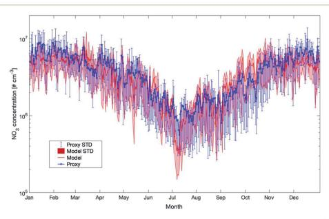
Fig. 14 Yearly mean daily time series of  $NO_3$  concentrations estimated by SOSAA (Model) and a proxy parameterization (Proxy) at 32.8 m based on the reference for the years 2007-2018 at SMEAR II (STD = standard deviation).
