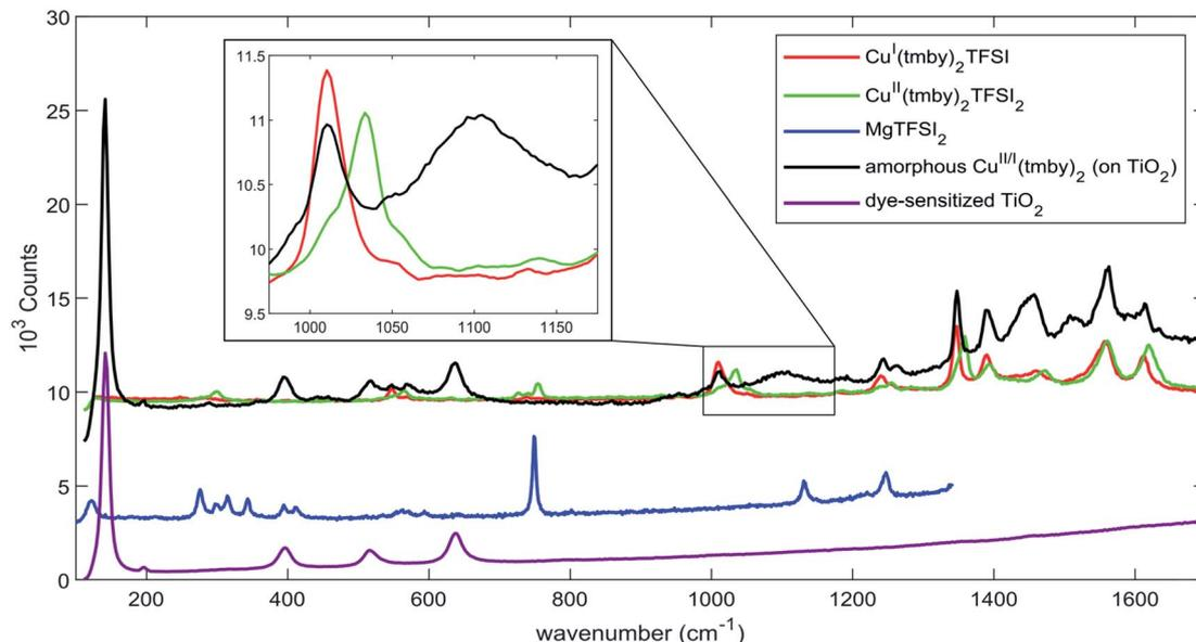
Fig. 4 Raman spectra of  $\text{Cu}^{\text{III}}(\text{tmby})_2 \text{TFSI}_{(2)}$  and  $\text{MgTFSI}_2$  (powders), DSCs sensitized with the XY1:L1 sensitizer combination as well as (sensitized) DSCs containing amorphous  $\text{Cu}^{\text{III}}(\text{tmby})_2 \text{TFSI}_{(2)}$  hole transport material. The two latter spectra were recorded inside the 'sandwich' DSC. Spectra are offset for clarity.
