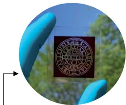
Dye-sensitized solar cells harvest energy from diffuse light with high efficiency.
