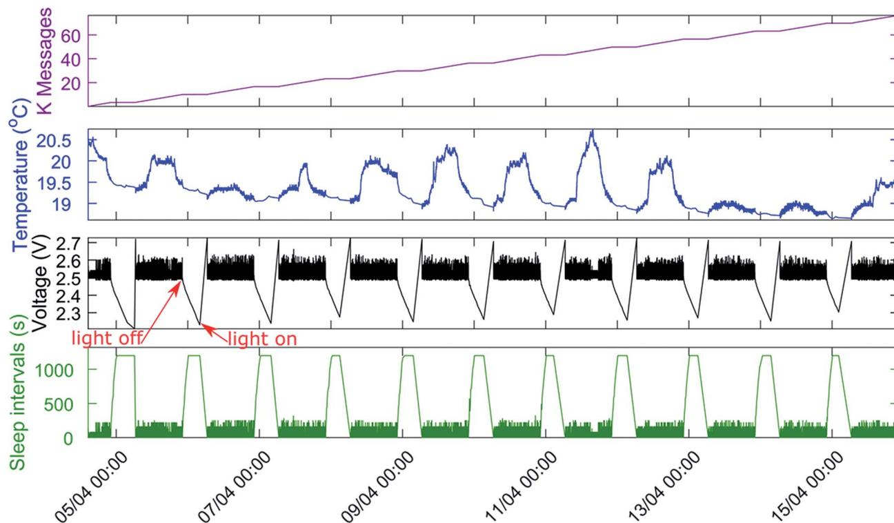
Fig. 6 Atmega328P-based wireless node equipped with transceiver and AVX 6.0 V 0.47 F supercapacitor. The sensor is powered by five serial 3.2 cm<sup>2</sup> photovoltaic cells (total 16.0 cm<sup>2</sup>). The sensor was tested in simulated light intervals of 16 hours "day" (1000 lux) and 8 hours darkness (10 pm–6 am, red arrows).
