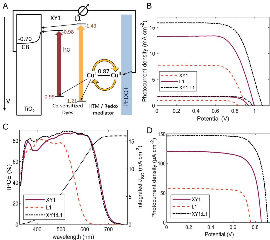
Fig. 2 (A) Working principle of the XY1:L1-sensitized DSC. (B) Photovoltaic performance under simulated sunlight (AM 1.5G,  $100 \text{ mW cm}^{-2}$ ) and 10% sunlight, (C) incident photon to current conversion efficiency spectra (IPCE), and (D) photovoltaic performance under 1000 lux fluorescent light ( $303.1 \mu\text{W cm}^{-2}$ ) of XY1, L1 and XY1:L1 co-sensitized DSCs. Corresponding parameters are listed in Table 1.
