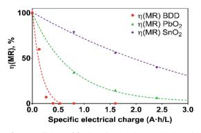
Fig. 7 Current efficiency ( $\eta$ ) values for the electrooxidation of MR as a function of the specific electrical charge (A h L<sup>-1</sup>) for solutions containing 20 mg L<sup>-1</sup> MR in 0.5 M H<sub>2</sub>SO<sub>4</sub> at 30 mA cm<sup>-2</sup> and 298 K: • Si/BDD, • Ti/Sb-doped SnO<sub>2</sub>, • Pb/PbO<sub>2</sub>.
