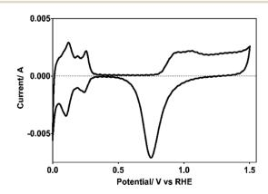
Fig. 1 Voltammogram of the Pt electrode used as cathode, recorded in  $0.5 \, \text{M} \, \text{H}_2 \text{SO}_4$  as supporting electrolyte at  $v = 50 \, \text{mV} \, \text{s}^{-1}$  and at 298 K.
