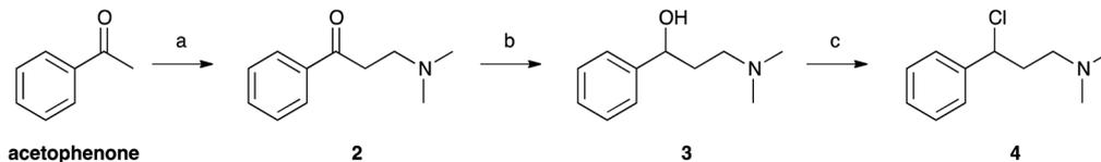
Scheme 1 (a) dimethylamine HCl/HCOH/EtOH; (b) NaBH<sub>4</sub>/KOH/MeOH; (c) SOCl<sub>2</sub>.
