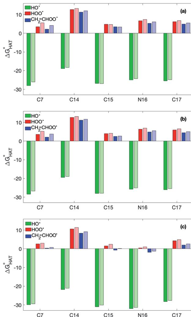
Fig. 3  $\Delta G_{\text{HAT}}^{\circ}$  (kcal mol<sup>-1</sup>) in the gas phase (a), in benzene (b), and in water (c) for the scavenging of HO<sup>•</sup>, HOO<sup>•</sup> and CH<sub>2</sub>=CHO<sup>•</sup> from non-aromatic sites of selenofluoxetine. Values for fluoxetine taken from Muraro *et al.*<sup>17</sup> are showed in a lighter shade for comparison. Level of theory: (SMD)-M06-2X/6-311+G(d,p)//M06-2X/6-31G(d).
