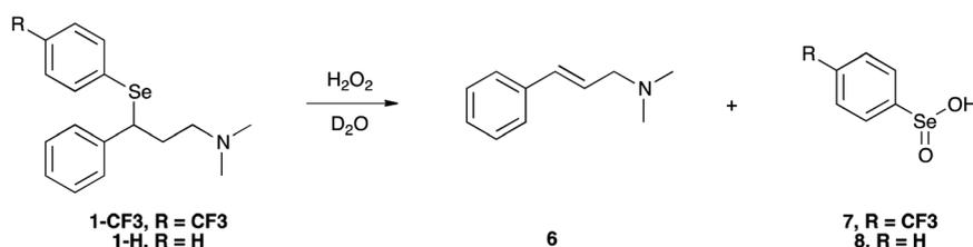
Scheme 3 Oxidation of **1-CF<sub>3</sub>** and **1-H** by H<sub>2</sub>O<sub>2</sub>. This scheme represents the overall reaction leading to the formation of cinnamylamine and seleninic acid, which were experimentally observed as final products.
