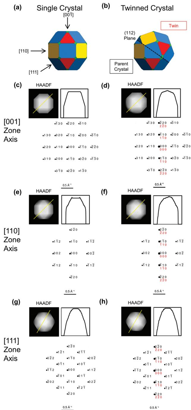
**Fig. 2** Simulated images and diffraction patterns for BCC single crystal (left) and twinned NPs (right) from Fig. 1b and c, reproduced in (a and b). (c–h) Projected thickness maps as a proxy for HAADF-STEM images, thickness profile along the yellow line, and simulated diffraction patterns, with parent in black and twin in red. Diffraction spots areas scale with intensity.
