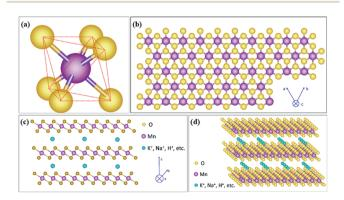
Fig. 1 (a) MnO<sub>6</sub> octahedron unit; (b) schematic diagram of birnessite along the 001 plane; (c) schematic diagram of birnessite viewed along the 011 plane; (d) stereoscopic schematic diagram of birnessite.
