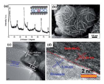
Fig. 2 (a) Typical XRD pattern of birnessite. 65 (b) SEM image of typical birnessite.<sup>67</sup> (c) and (d) HRTEM images of typical birnessite.<sup>49,68</sup>
