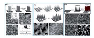
Fig. 12 (a) Co<sub>3</sub>O<sub>4</sub> nanowire@birnessite ultrathin nanosheet core/shell arrays.155 (b) Co<sub>3</sub>O<sub>4</sub>@birnessite hierarchical nanoneedle arrays.167 (c) Hierarchical Co<sub>3</sub>O<sub>4</sub>@birnessite core-shell arrays.<sup>68</sup>
