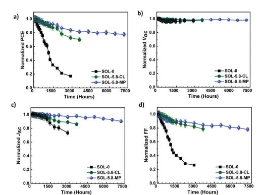
Fig. 5 Evolution of J-V parameters (a) PCE, (b)  $V_{oc}$ , (c)  $J_{sc}$ , and (d) FF for the different devices measured at different periods over ten months. Devices are always stored and measured under ambient laboratory conditions (T = 22-25 °C, and RH = 25-55% RH).
