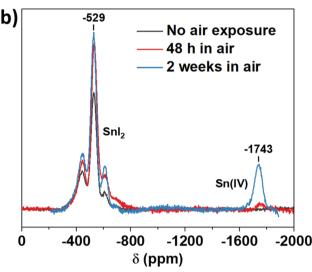
Fig. 1 (a) Steps of tin-based perovskite material preparation studied in this work as possible sources of Sn(II) oxidation; (b) solid-state 119Sn-NMR spectra of Snl<sub>2</sub> precursor with and without air exposure.
