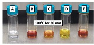
Fig. 3 (a)  $^{1}$ H-NMR spectra of FASnl $_{3}$  and MASnl $_{3}$  in DMSO at 1 M after heating the solutions at 100  $^{\circ}$ C for 30 min. The green arrow highlights the peak of DMS originating from heating the solution; (b) vials containing different solutions before and after being heated at 100  $^{\circ}$ C for 30 min. A: FAI in DMSO; B: Snl $_{2}$  in DMSO; C: FASnl $_{3}$  in DMF; D: FASnl $_{3}$  in DMSO with 10 mol% SnF $_{2}$ ; E: CsSnl $_{3}$  in DMSO.
