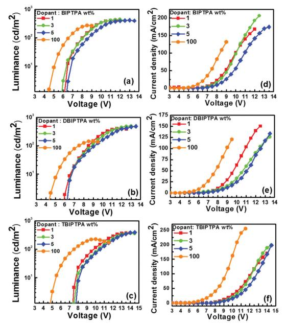
Fig. 9 Luminance-current density (a-c) and current density-voltage (d-f) plots of the solution-processed OLED devices with BIPTPA, DBIPTPA and TBIPTPA dopants at various concentrations in the CBP host.
