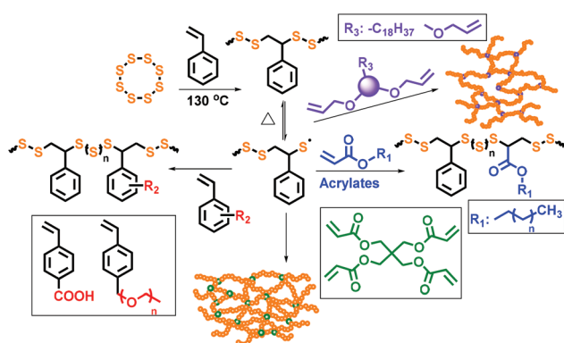
Fig. 25 Dynamic covalent polymerization of poly( S-r-Sty ) with acrylates, functional styrenes and an acrylic crosslinker. Reproduced with permission from ref. 52. Copyright 2017 The Royal Society of Chemistry.
