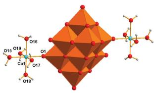
Fig. 1 Molecular structures of the anions  $[\{Cu(H_2O)_2(2-hep)\}_2V_{10}O_{28}]^2$  $(V_{10}Cu)$  and  $[\{Co(H_2O)_5\}_2V_{10}O_{28}]^{2-}$   $(V_{10}Co)$  as revealed by X-ray crystallography showing atom labelling. Colour code: orange octahedra {VO<sub>6</sub>}, green Cu, light blue Co, blue N, red O, black C, gray H. Ellipsoids are displayed at a 30% probability level.
