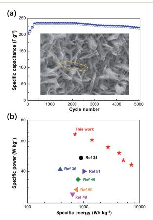
Fig. 9 (a) Cycle life and SEM images of the assembled ZNGN//AC device for 5000 cycles, (b) Ragone plot of the device assembled using the dual-morphology  $\rm ZnCo_2O_4$  when compared with the recently reported values in the literature. The crack produced after 5000 cycles is highlighted by the yellow dotted circle in (a).
