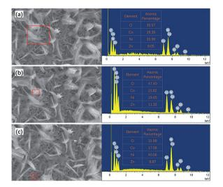
Fig. 5 EDS results of (a) dual-morphology  $ZnCo_2O_4$ , (b) feather-like  $ZnCo_2O_4$ , and (c)  $ZnCo_2O_4$  nanosheet .
