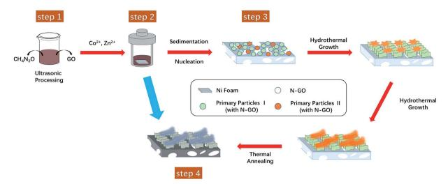
Fig. 6 Schematic of the fabrication process of the 3D hierarchical dual-morphology ZnCo<sub>2</sub>O<sub>4</sub> on NF.
