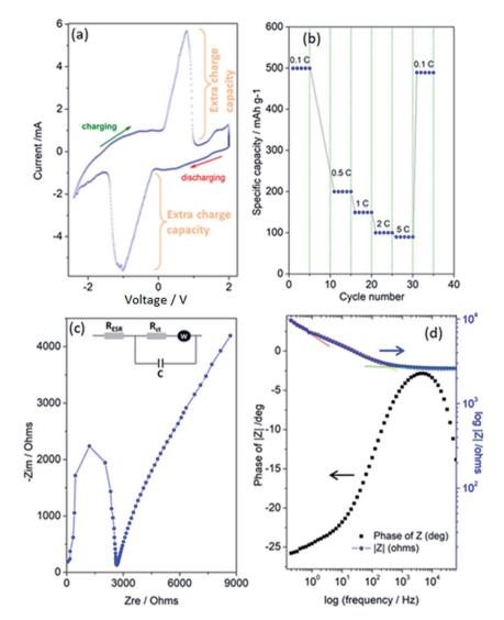
Fig. 5 Electrochemical performance results of the *superbat* designed with ZnO nanocrystal and graphene foam electrodes, LiPF<sub>6</sub> electrolyte, and a glass fiber separator. (a) Cyclic voltammetry (CV), (b) rate performance obtained from the galvanostatic cycle with potential limitation (GCPL) technique. (c) Nyquist plot and (d) Bode plot obtained from electrochemical impedance spectroscopy (EIS).
