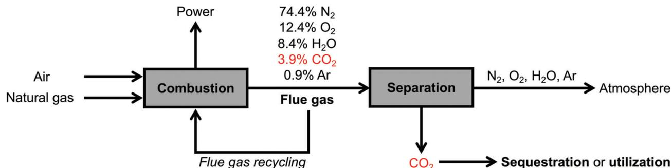
Fig. 2 Schematic of a natural gas-fired power plant with post-combustion CO<sub>2</sub> capture, including optional flue gas recycling to increase the concentration of CO<sub>2</sub> in the flue gas up to ~8%.
