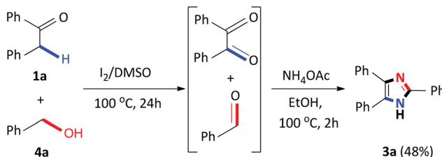
**Scheme 4** Domino convergent synthesis of 2,4,5-triphenyl imidazole **3a**.
