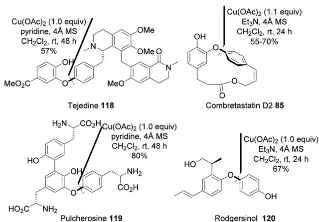
**Fig. 4** Application of the intermolecular Chan–Lam–Evans reaction in natural product synthesis.
