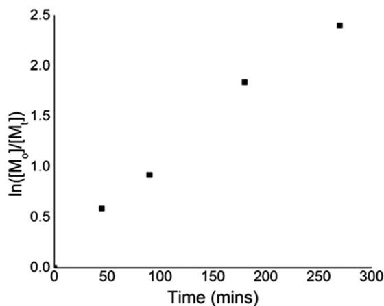
Fig. 3 Kinetic plot for the polymerization of metal-free ATRP using eosin Y.
