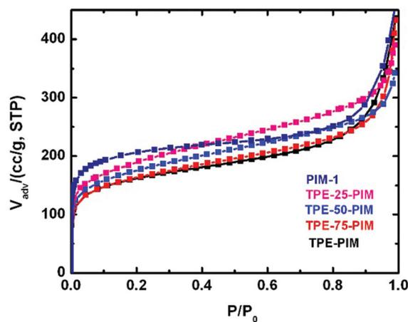
Fig. 4 N<sub>2</sub> adsorption isotherms of the TPE-Based PIMs and PIM-1 at -196 °C.
