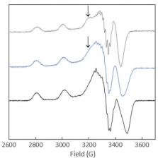
Fig. 4 EPR spectra of Cu(II) –  $A\beta ox$  (blue curve), Cu(II) –  $A\beta_{28}$  (black curve) and Cu(II)-AcAβ<sub>28</sub> (grey curve) at pH 12.5. Aqueous solution with 10% of glycerol containing  $^{65}$ Cu (450  $\mu$ M) and peptide (500  $\mu$ M). T = 120 K,  $\nu$  = 9.5 GHz, microwave power = 20.5 mW, amplitude modulation = 10.0 G, and modulation frequency = 100 kHz.
