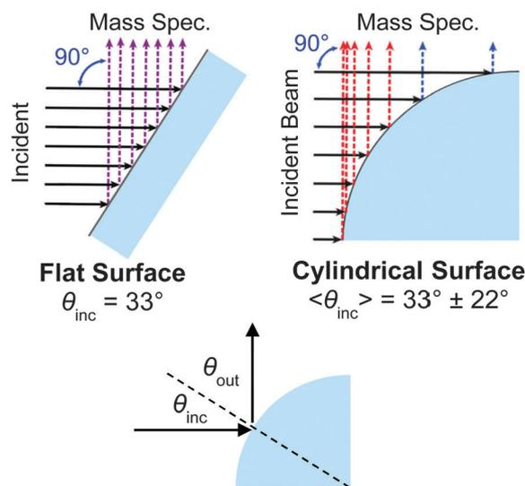
Fig. 6 Comparison of trajectories scattering from a cylindrical jet and a flat film at a deflection angle of 90°. The flat film is tilted at the average incident angle of 33° intercepted by the cylinder.
