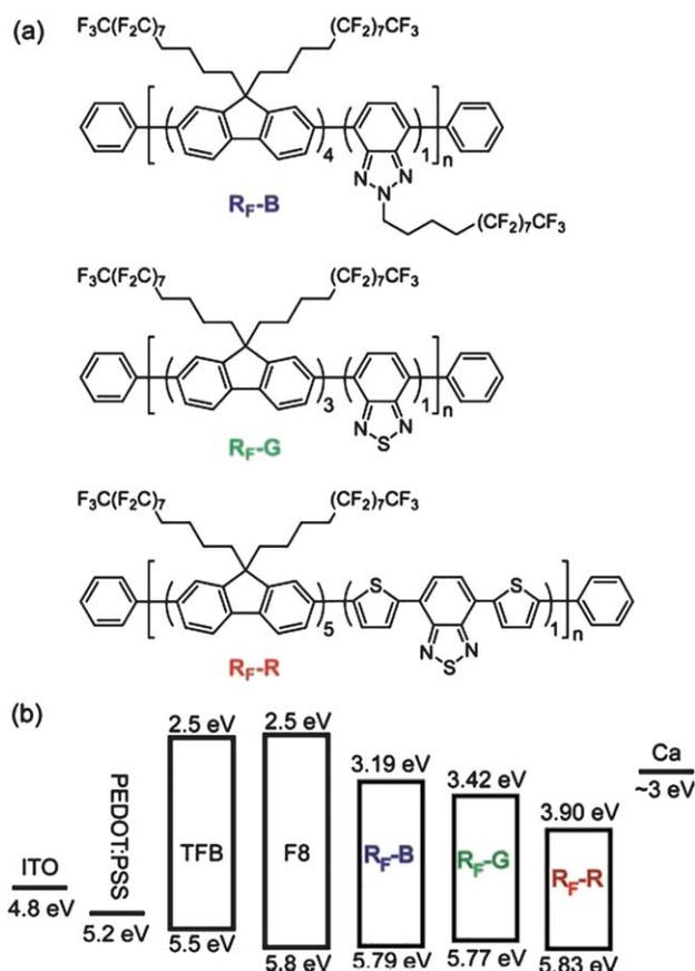
**Fig. 3** (a) Polymer structures of **RF-B**, **RF-G**, and **RF-R** polymers. (b) The energy diagram of ITO, PEDOT:PSS, poly[(9,9-dioctylfluorene)-*co*-(4-butylphenyl)diphenylamine] (**TFB**), Poly(9,9-dioctylfluorene) (**F8**), **RF-B**, **RF-G**, **RF-R**, and Ca. Adapted with permission from ref. 156, Copyright 2010 Wiley-VCH Verlag GmbH & Co. KGaA.
