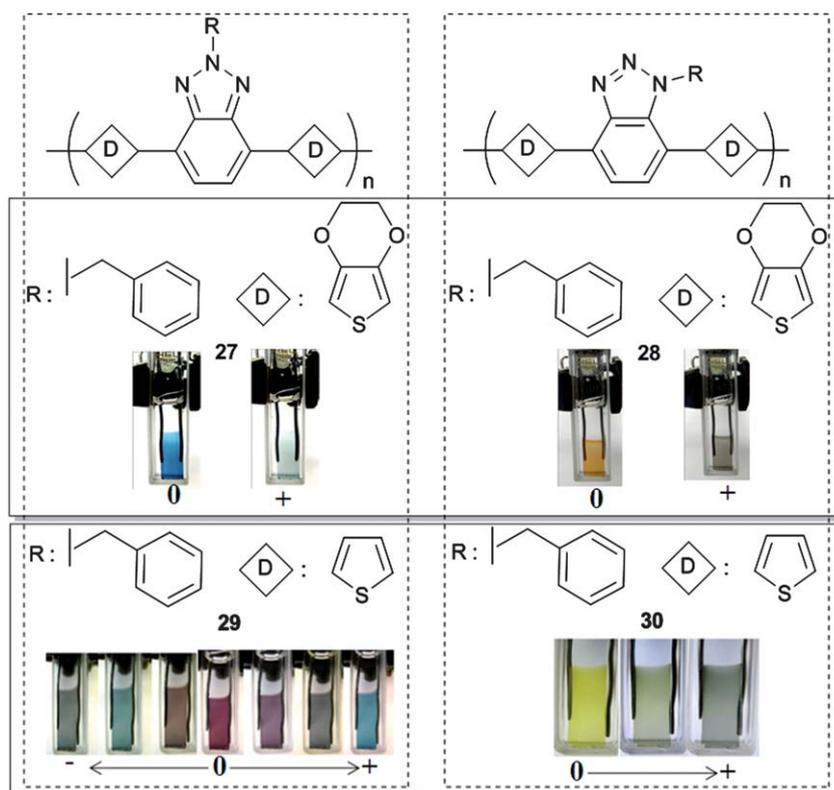
**Fig. 2** Chemical structures of D–A type BTz polymers and their colors in neutral, oxidized and reduced states. **27, 28** Adapted with permission from ref. 55, Copyright 2010 Elsevier B. V.; **29, 30** Adapted with permission from ref. 58, Copyright 2010 Elsevier B. V.
