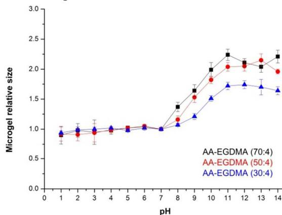
**Figure 5.** Swelling ratios of the AA-EGDMA microgels in different pH environments. Microgels formed from THPA:EGDMA molar ratios of 70:4, 50:4 and 30:4 are represented as squares, circles and triangles, respectively.
