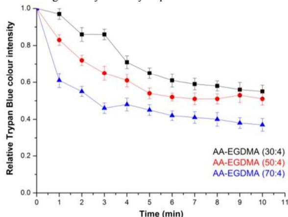
**Figure 9.** Hydrophilic dye release in basic pH solution (~pH 8.5). The plots show the relative Trypan Blue colour intensity versus time for all three types of AA-EGDMA microgels with different crosslinking densities. Squares, circles and triangles represent the 70:4, 50:4 and 30:4 AA:EGDMA molar ratios, respectively.
