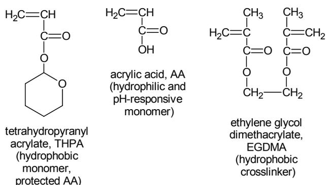
**Figure 1.** Chemical structures of the monomers and crosslinker.
