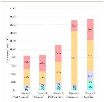
Fig. 1 Net removal costs categorized by process stages for 5 key
