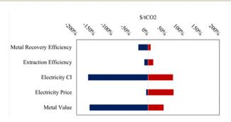
Fig. 5 Sensitivity analysis on net storage cost coupled to pH-swing critical
