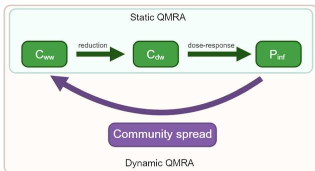
**Fig. 6** Differences between dynamic and static QMRAs.  $C_{ww}$  is the pathogen concentration in wastewater.  $C_{dw}$  is the pathogen concentration in drinking water.  $P_{inf}$  is the probability of infection.
