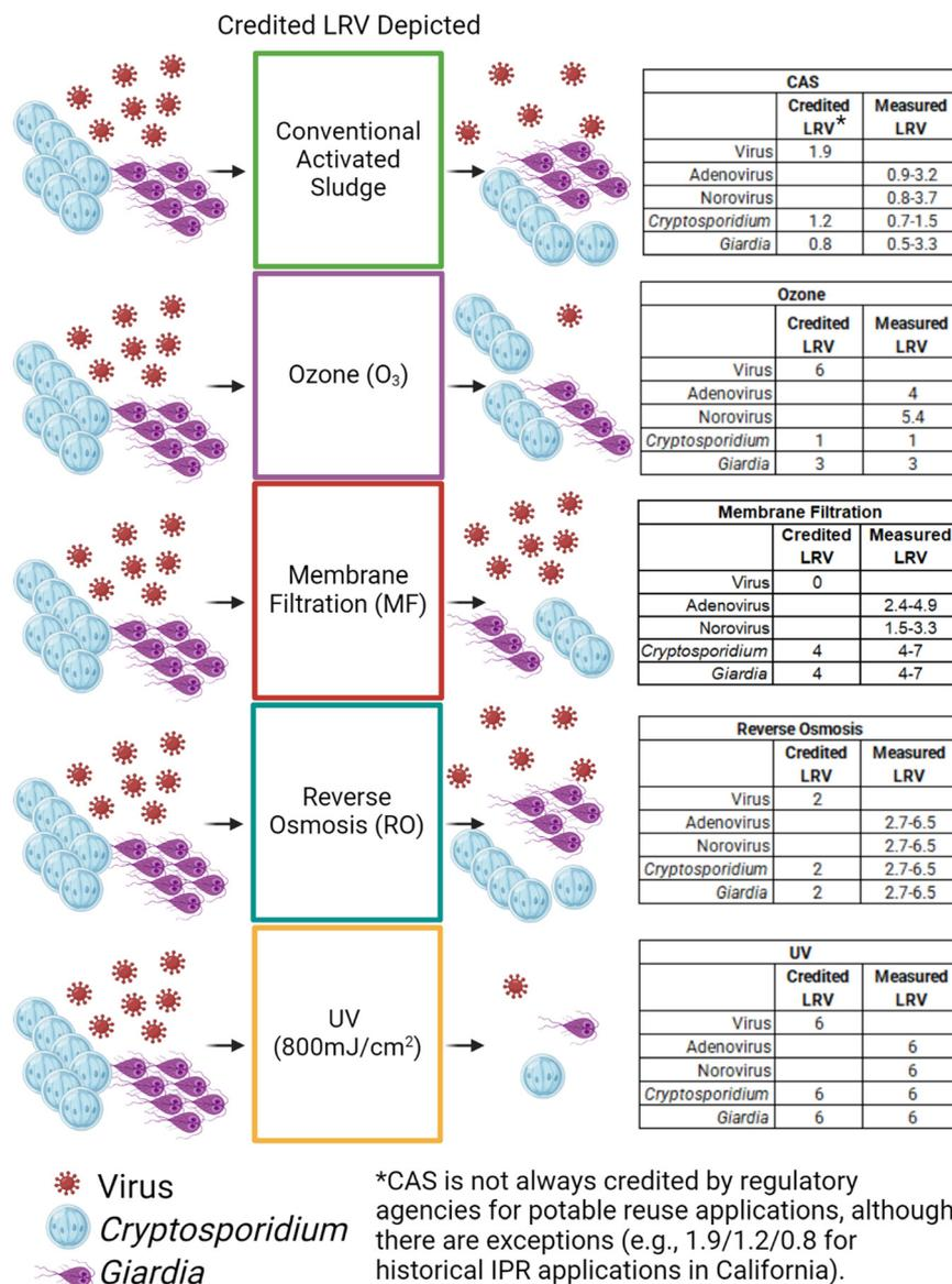
Fig. 4 Conceptual diagram of the credited effectiveness of different treatment processes on protozoa and viruses. LRVs from Soller *et al.*<sup>45</sup> Note that observed treatment efficacy may be substantially different from credited treatment efficacy, resulting in an LRV 'gap'.
