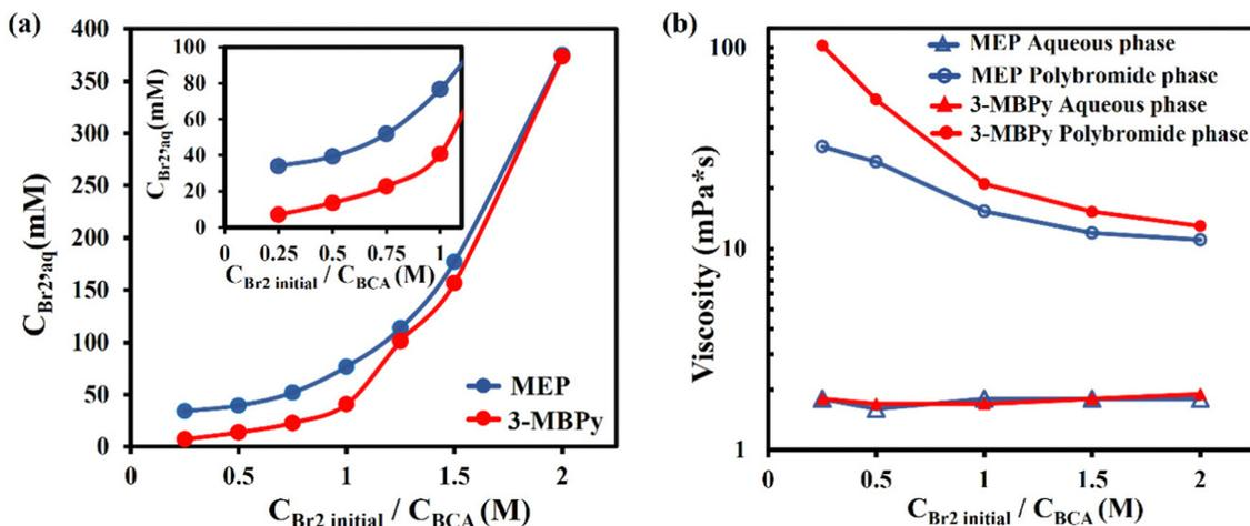
Fig. 3 *Ex situ* characterization of electrolytes containing initial (pre-partition) bromine concentration ranging from 0.25 M to 2 M, as well as 2 M  $\text{ZnBr}_2$ , and 0.5 MEP or 3-MBPY. (a) Measured bromine concentration in the aqueous phase at equilibrium, versus initial bromine concentration. (b) Measured viscosity of each phase versus initial bromine concentration.
