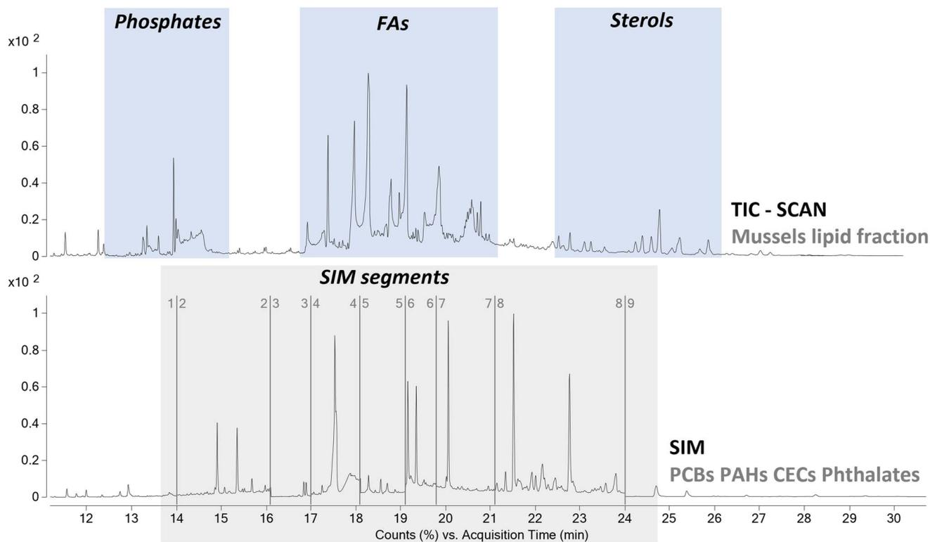
**Fig. 2** Py-GC-MS chromatogram obtained for the mussels spiked with the standard solution of pollutants at the best extraction conditions; total ion chromatogram (TIC), above; selected ion monitoring (SIM) chromatogram, below.
