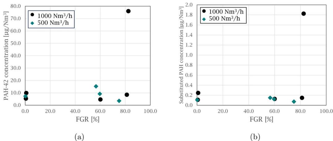
Fig. 6 Graphs showing the estimated PAH stack emissions for PAH-42 and substituted PAHs (sum of oxy- and nitro-PAHs) for both 1000 Nm<sup>3</sup> h<sup>-1</sup> and 500 Nm<sup>3</sup> h<sup>-1</sup> at varying FGR levels. (a) PAH-42 and (b) substituted PAH.
