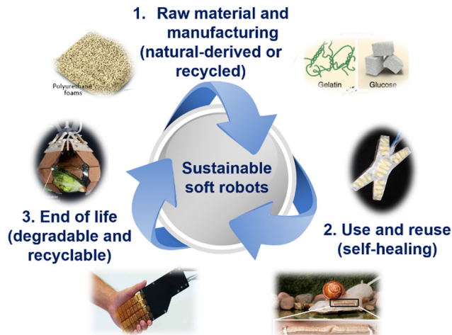
Fig. 1 The life cycle assessment of sustainable soft robots. Three main phases are classified from cradle to grave. Raw materials that are natural or recycled and manufacturing encode the original sustainable character at the start-of-life. Self-healing enables to reuse and refunction from damage at the middle-of-life. Degradable and recyclable allows degradation and recycle into a new life at the end-of-life instead of being discarded directly. Reproduced from ref. 4; Copyright 2023, Springer Nature. Reproduced from ref. 5; Copyright 2020, Springer Nature. Reproduced from ref. 6; Copyright 2022, the American Association for the Advancement of Science. Reproduced from ref. 7; Copyright 2023, Springer Nature. Reproduced from ref. 8; Copyright 2023, the American Association for the Advancement of Science. Reproduced from ref. 9; Copyright 2017, the American Association for the Advancement of Science.
