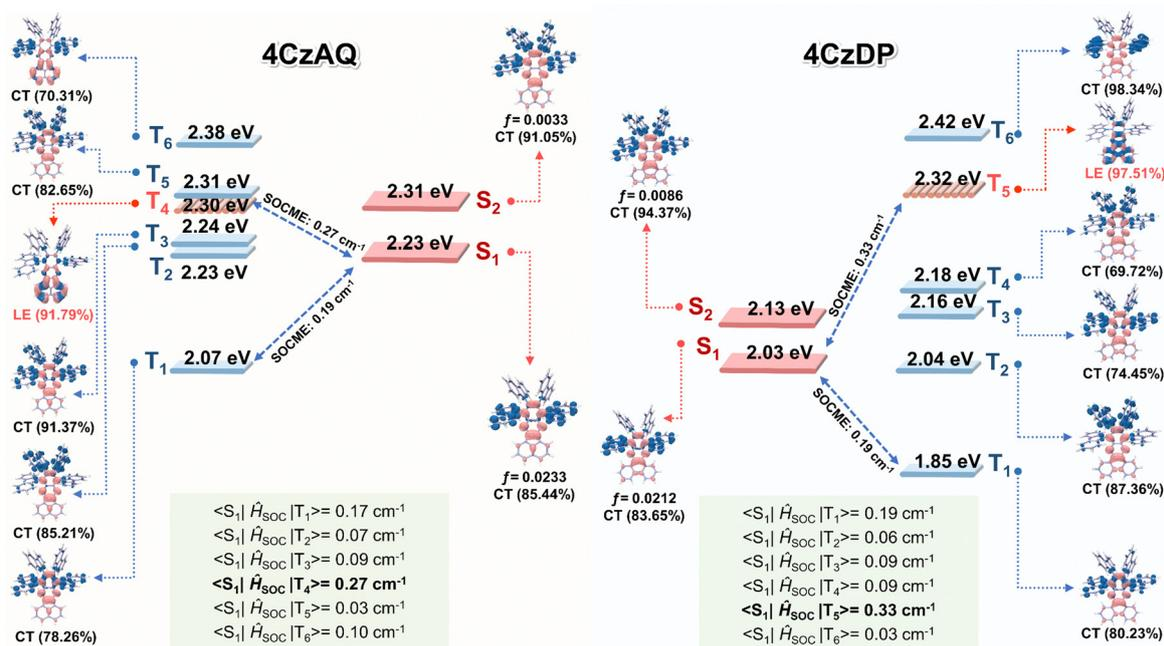
Fig. 4 Energy-level diagram with NTOs for the excited singlet ( $S_n$ ) and triplet ( $T_m$ ) states (Hole: blue color; particle: pink color), and SOC matrix elements between the  $T_m$  and  $S_n$  states of **4CzAQ** and **4CzDP**.
