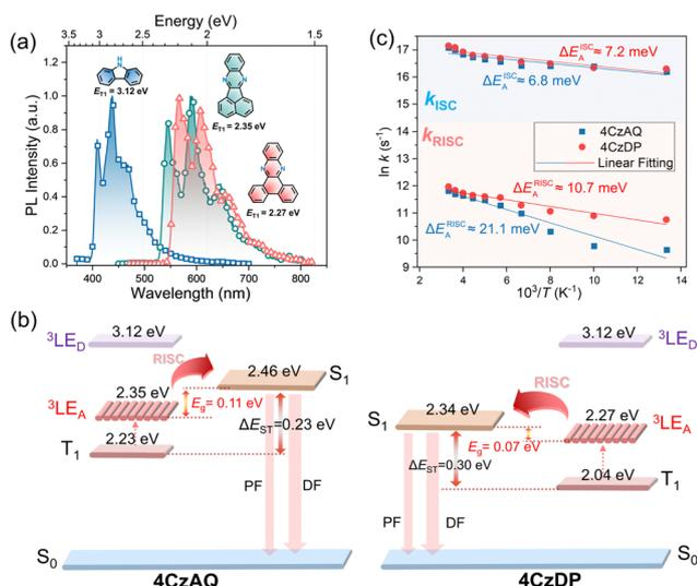
Fig. 6 (a) Phosphorescence spectra of AQ, PQ and carbazole (Cz) fragments with a delay of 10 ms at 77K; (b) temperature dependences of  $k_{\text{ISC}}$  and  $k_{\text{RISC}}$  for the 10 wt% TADF-emitter-doped CBP films ( $E_{\text{A}}$  is calculated according to the Arrhenius equation); (c) the schematic diagram of the exciton dynamic process of **4CzAQ** and **4CzDP**.
