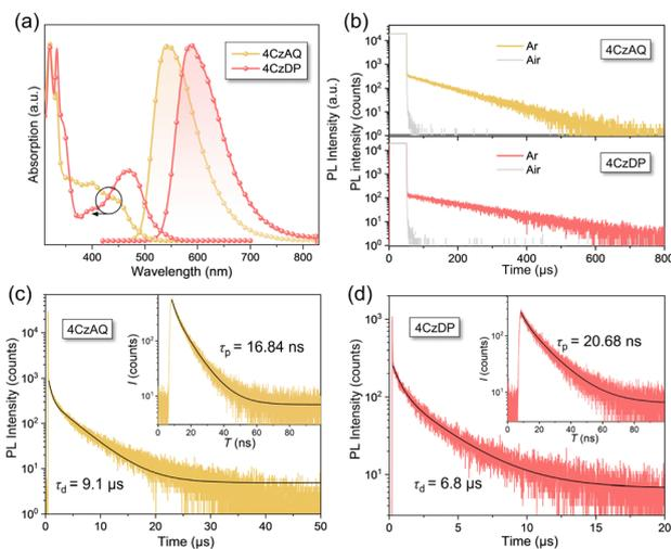
Fig. 5 (a) UV-vis absorption and PL spectra of **4CzAQ** and **4CzDP** in toluene ( $10^{-5}$  mol  $\text{L}^{-1}$ ); (b) Transient PL decay curves of **4CzAQ** and **4CzDP** in toluene ( $10^{-5}$  mol  $\text{L}^{-1}$ ) before and after Ar bubbling; (c) Transient PL decay curve of 10 wt% **4CzAQ**-doped CBP films at 300 K under a nitrogen atmosphere; (d) Transient PL decay curve of 10 wt% **4CzDP**-doped CBP films at 300 K under a nitrogen atmosphere.
