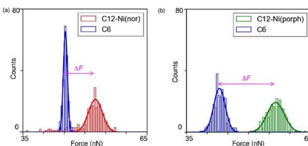
**Fig. 3** Histograms of the observed adhesive force constructed from the 256 force curves for (a) the C6 matrix with and without C12-Ni(nor) and (b) the C6 matrix with and without C12-Ni(porph). The bold lines are the result of the Gaussian fitting of the histograms.  $\Delta F$  is the difference between peak adhesion forces for C6 and C12-Ni(nor) or C6 and C12-Ni(porph).
