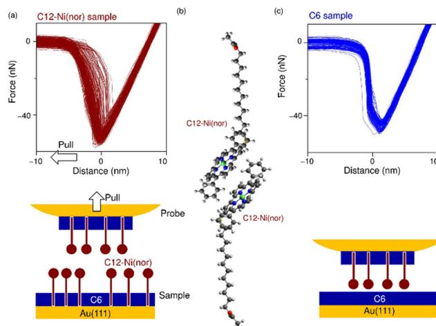
**Fig. 2** (a) and (c) Force curves measured on the C6 matrix with and without C12-Ni(nor). Adhesion force was defined as the maximum attraction (most negative force signal value) measured by the force curve. Schematics of the experimental systems are shown at the bottom. (b) Schematic illustration of the  $\pi$ -stack formation between C12-Ni(nor) molecules. Grey, white, blue, red, yellow, and green balls correspond to C, H, N, O, S and Ni atoms, respectively.
