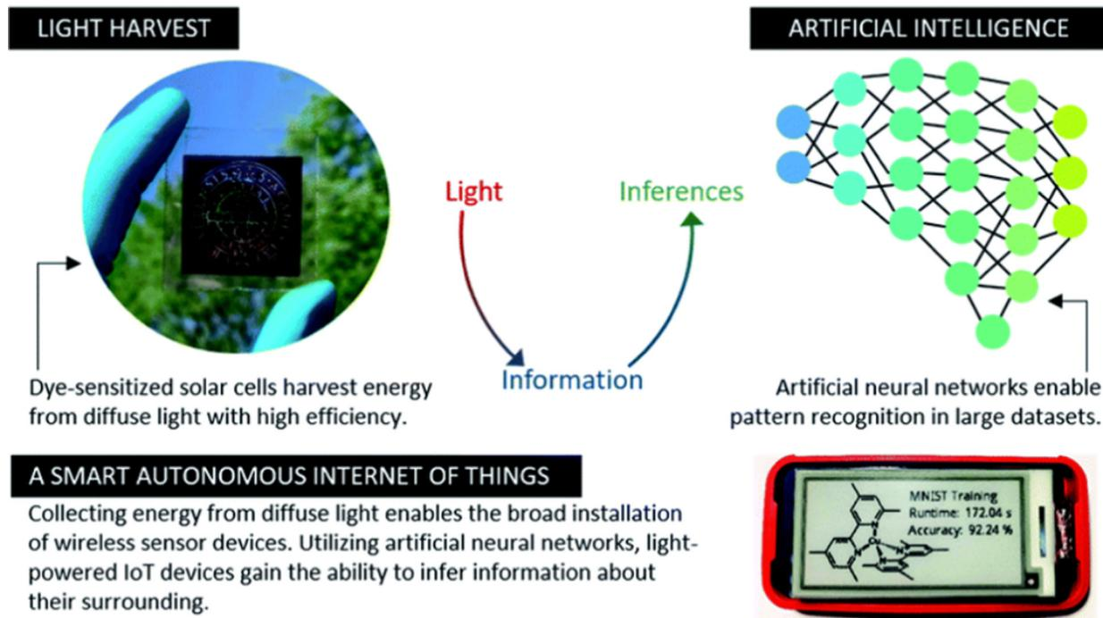
Fig. 13 Fully autonomous IoT devices powered by harvested ambient light directly convert photons into computational information. Reproduced with permission of ref. 9 (Licensed Under a Creative Commons Attribution 3.0 Unposter Licence).
