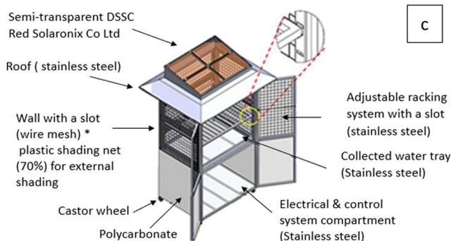
Fig. 12 (a) and (b) DSSM application in an Aquaponic greenhouse.<sup>17</sup> (c) The detailed construction drawings of PDMG prototype. Reproduced with permission ref. 233 Elsevier.
