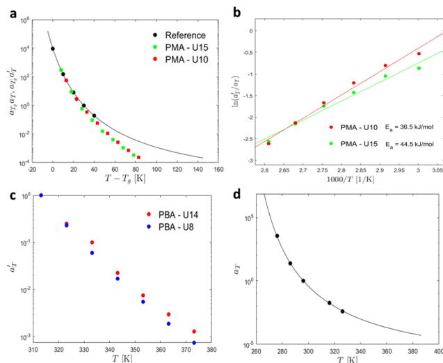
**Fig. 17** (a) Shift factors of PMA-U15, PMA-U10, and the reference at  $T_{\text{ref}} = 40$  °C. (b) Extraction of the activation energy of PMA-U15 and PMA-U10. (c) Shift factors of PBA-U9 and PBA-U14 at  $T_{\text{ref}} = 40$  °C. (d) Shift factors of PBA at  $T_{\text{ref}} = 30$  °C. The black line corresponds to the prediction of the WLF equation.
