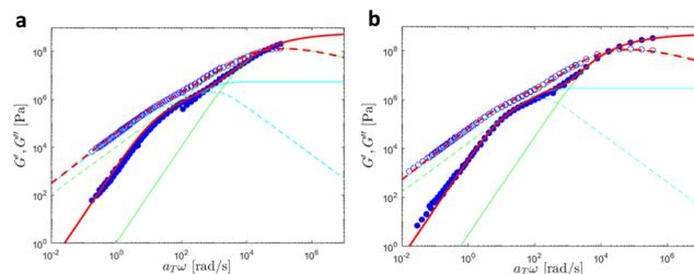
Fig. 15 Linear viscoelastic mastercurves of (a) PMA at  $T_{ref} = 30$  °C and (b) PBA at  $T_{ref} = -30$  °C. Red lines correspond to the model predictions obtained with the values shown in Tables 1 and 2. The contributions from the KWW model (in green) and the Rouse model (in cyan) are also presented.
