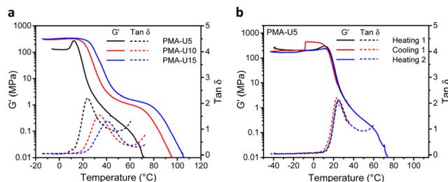
Fig. 8 DMTA curves of the PMA-UPy networks. (a) Storage modulus ( $G'$ ) and loss factor ( $\tan \delta$ ) as a function of temperature for all polymers; (b) storage modulus ( $G'$ ) and  $\tan \delta$  as a function of temperature for a second sample of PMA-U5 in two heating runs and one cooling run. Note that the absolute  $G'$  values are lower than expected for glassy polymers indicating that the calibration was not optimal, which will, however, not influence the relative trends.
