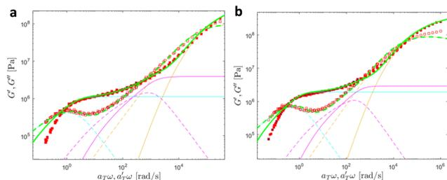
**Fig. 18** Linear viscoelastic mastercurves of (a) PMA-U10 and (b) PMA-U15 at  $T_{\text{ref}} = 70$  °C. Green corresponds to the model predictions obtained with the parameters shown in Tables 1 and 2. The contributions from the KWW model (in orange), the Rouse model (in magenta), and the slow modes (in cyan) are also presented.
