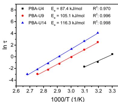
Fig. 14 Arrhenius plot of the relaxation times for the PBA–UPy networks, determined by the crossover points of  $G'$  and  $G''$  in the frequency sweeps with apparent activation energy ( $E_a$ ) obtained by linear fitting of the data.
