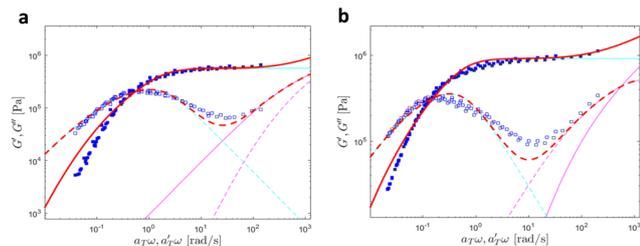
Fig. 19 Linear viscoelastic mastercurves of (a) PBA-U8 and (b) PBA-U13 at  $T_{\text{ref}} = 40$  °C. Red lines correspond to the model predictions obtained with the values shown in Tables 1 and 2. The contributions of the Rouse model (in magenta) and the slow modes (in cyan) are also presented.
