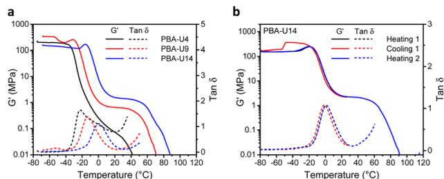
Fig. 12 DMTA curves of the PBA-UPy networks. (a) Storage modulus ( $G'$ ) and loss factor ( $\tan \delta$ ) as a function of temperature for all polymers; (b) storage modulus ( $G'$ ) and  $\tan \delta$  as a function of temperature for a second sample of PBA-U14 in two heating runs and one cooling run. Note that the absolute  $G'$  values are lower than expected for glassy polymers indicating that the calibration was not optimal, which will, however, not influence the relative trends.
