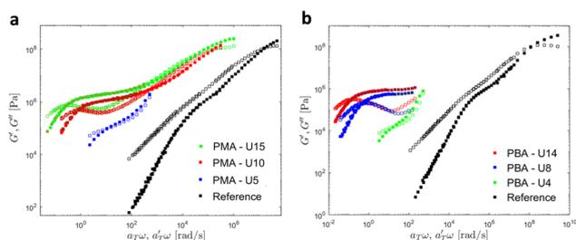
**Fig. 16** Pseudo-mastercurves, mastercurve or curves of (a) PMA systems at  $T_{\text{ref}} = 70$  °C and of (b) PBA systems at  $T_{\text{ref}} = 40$  °C. The mastercurves of the references were shifted using the WLF equation (see eqn (1)).
