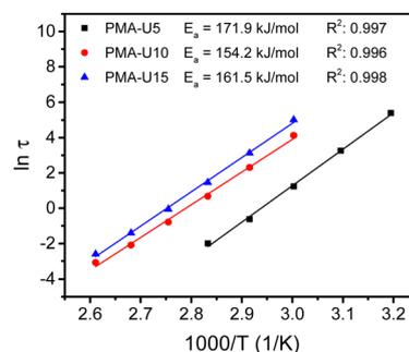
Fig. 10 Arrhenius plot of the relaxation times for the PMA-UPy networks, determined by the crossover points of  $G'$  and  $G''$  in the frequency sweeps with apparent activation energy ( $E_a$ ) obtained by linear fitting of the data.
