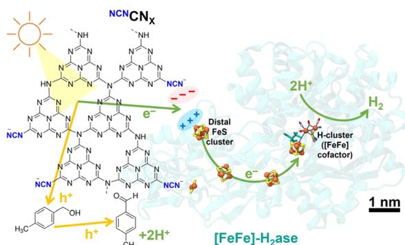
**Fig. 1** Schematic of photocatalytic H<sub>2</sub> evolution coupled with alcohol oxidation to aldehyde using an electrostatic <sup>NCN</sup>CN<sub>x</sub>||[FeFe]-H<sub>2</sub>ase (CpI, PDB: 4XDC) assembly. Scale bar refers to enzyme and CN<sub>x</sub> is not shown to scale.
